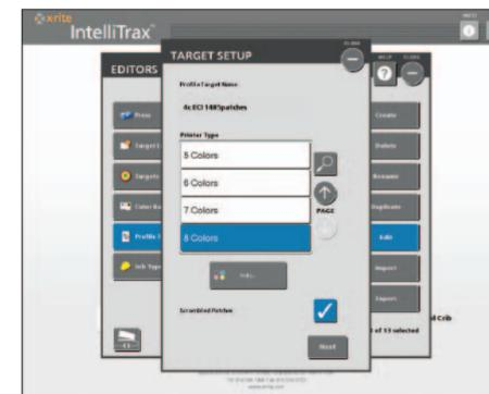
IntelliTrax ICC generates profiles for up to 8 ink colors all from a miniature test target no larger than a multi-tier color bar.
