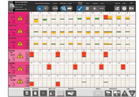
A special mode in IntelliTrax alerts operators to all color issues that exist within any given printing unit.
