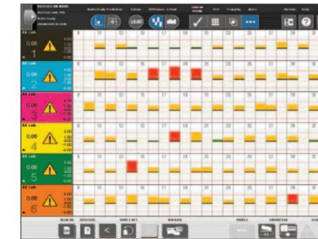
IntelliTrax has the power to evaluate industry standard color difference (ΔE) to ensure color matches customer specifications.
